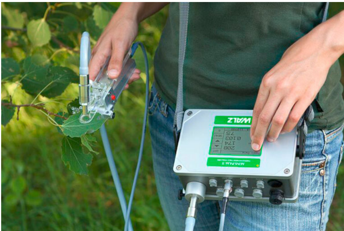
Measuring chlorophyll fluorescence with the MINI-PAM fluorometer
